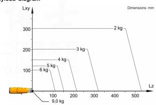
The KR 6 R1840-2 is designed for a rated payload of 6 kg in order to optimize the dynamic performance of the robot. With reduced load center distances, higher loads up to the maximum payload may be used. The specific load case must be verified using KUKA.Load. For further consultation, please contact KUKA Support.
